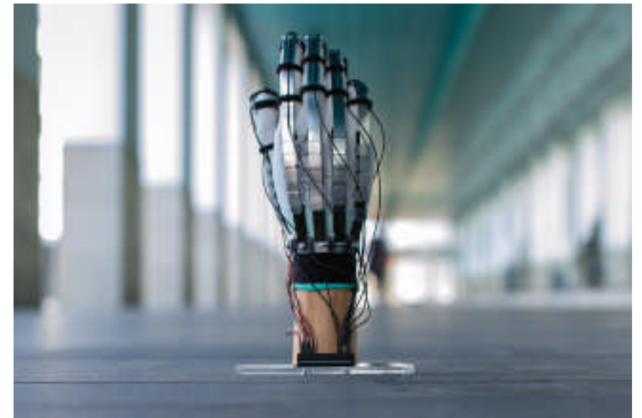
At present, the haptic glove draws power from a very thin cable.
