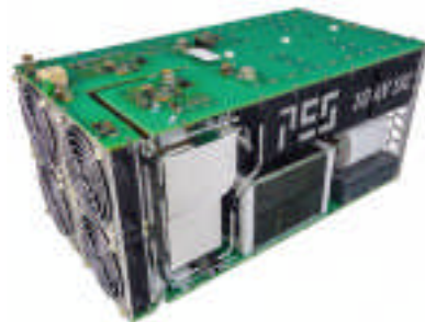
The medium-voltage converter is a component of the new smart transformer.
