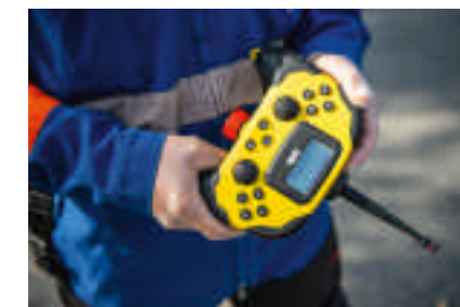
As a precautionary measure, an operator uses a joystick to take partial control of the robot’s first steps before switching to autonomous mode.
